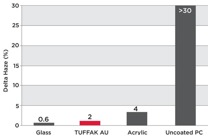
\*Taber Abrasion per ASTM D 1044, 100 cycles using CS-10F wheel
