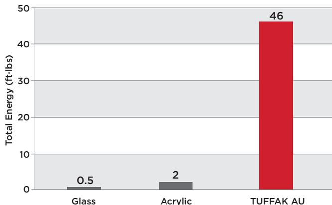
\*Instrumented Impact per ASTM D 3763, sample thickness is 0.125" nominal
